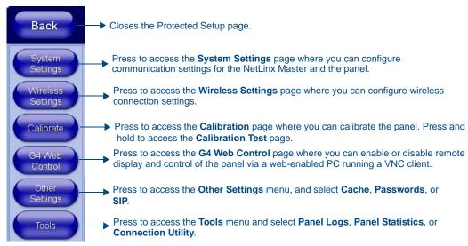
FIG. 49 Protected Setup Navigation Buttons (MVP-7500)
